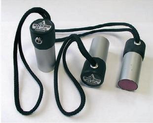
The device consists of an electronic unit with a display, where the results of testing are shown in the form of A-scan and a S0205 0.025A0D25CL low-frequency ultrasonic longitudinal wave transducer. The transducer is straight beam, single-crystal, broadband (relative bandwidth is not less than 100%) with liquid acoustic contact and working frequency of 25 kHz.
